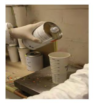
The first part of the mixing process is to pour out the required amount of shaken/stirred lacquer into the appropriate container.
