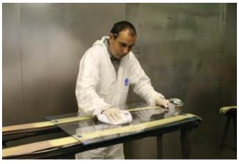
Before any spraying takes place it is very important to ensure that the glass is crystal clean and free from contaminates and particles.
