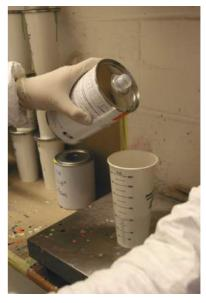
This can also be done by volume in a measuring jug or in a container with a measuring stick. It is imperative that the correct amount of hardener is put in as this affects the drying time, the adhesion, the gloss level and the elasticity and longevity of the product. Please refer to the TDS for the mixing ratio.
