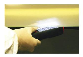
It is important to check that the finish is opaque. For this we recommend using a LED hand lamp which is put under the glass to check the opacity.
