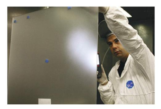
It is important to check that the finish is opaque. For this we recommend using a LED hand lamp which is put under the glass to check the opacity.
