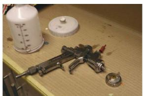
The first part of the mixing process is to pour out the stirred or shaken paint into the appropriate container. Mixing in the hardener can be done by weight on a set of scales.
