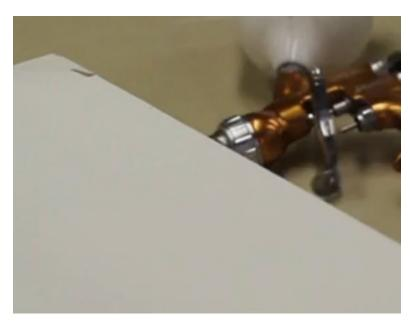
Apply two coats of AVKOTE SFP to the open edges. If it is good quality MDF you will probably only need one coat on the top face. MDF of a lesser grade will require two coats.
