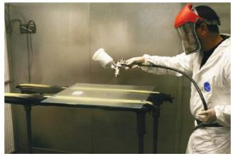
The problem with a metallic finish is that if you do not get an even coat, the aluminium particles in the paint will converge together and reflect the light in a way that will look like dark wavy lines in the finish. The way to stop this is to make sure that your gun is set right so that the paint is atomising correctly with the paint flow set low. This will allow you to put 2-4 coats on lightly but evenly.
