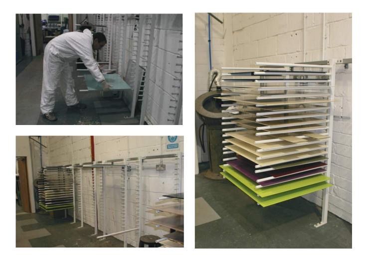
This can now be left to chemically cure for 24 hrs. It will cure from 8-10 degrees and above. At 20 degrees it will be 70% cured in about an hour and will be dry enough to handle.
