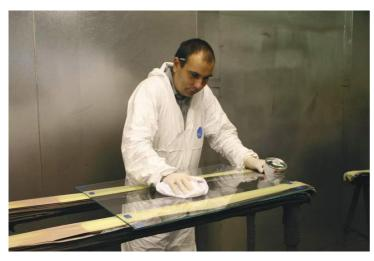
Before any spraying takes place it is very important to ensure that the glass is crystal clean and free from contaminates and particles.
