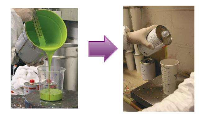
This can also be done by volume in a measuring jug or in a container with a measuring stick. It is imperative that the correct amount of hardener is put in as this affects the drying time, the adhesion, the gloss level and the elasticity and longevity of the product. Please refer to the TDS for the mixing ratio. When the paint is ready for spraying, pour it into your spray gun using an appropriate paint filter. Please note that the sparkle clear coat is not to be filtered.
